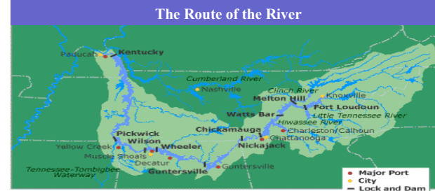
The River's main navigable channel is 652 miles long. It officially begins a mile above Knoxville, TN and eventually empties into the Ohio River at Paducah, KY. Commercial navigation also extends into three tributaries: 61 miles up the Clinch River, 29 miles up the Little Tennessee, and 21 miles up the Hiwassee River. Another 150 miles of channel—too shallow for commercial traffic—is marked for recreational use.
